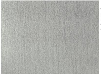
The image shows the surface of the Paran-S and the open structure is clearly visible.
