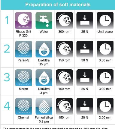
The parameters in the preparation method are based on 300 mm dia. disc size and 30 mm dia. individual samples
