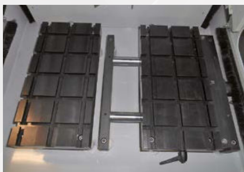
Transversal table X axis 120 mm stroke
