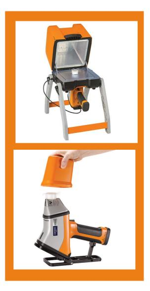
The sample is placed in a sample cup prepared with 3.5µm Mylar® film. Black mass is a low-density sample which scatters X-rays. Therefore, suitable radiation safety accessories, such as the light stand and safety shield or the benchtop stand must be used for the analysis. It is good practice to check the analyzer's protective window for contamination, and change it if contamination is suspected.
