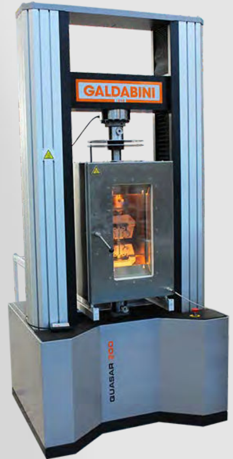
Universal testing machine Quasar 200 with Micron Motor MFX extensometer and thermostatic chamber
