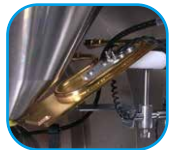
Cold trap – adapted to installation
