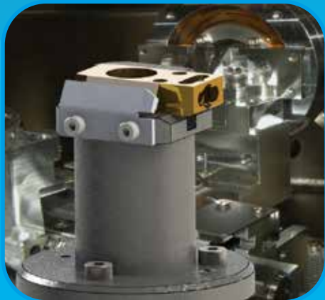
SEM stage and specimen shuttle
