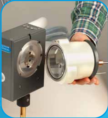
Vacuum/inert gas transfer device and airlock
