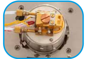
Nitrogen gas cooled stage
