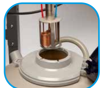
Heat exchanger and dewar
