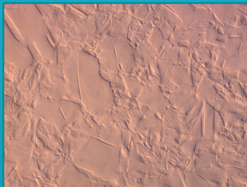
Copper, DIC, 200x after polishing with Fumed Silica, Alkaline, with additives, on Chemal.
