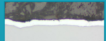
Zinc coating on steel, BF, 500x after polishing with Fumed Silica, WF.
