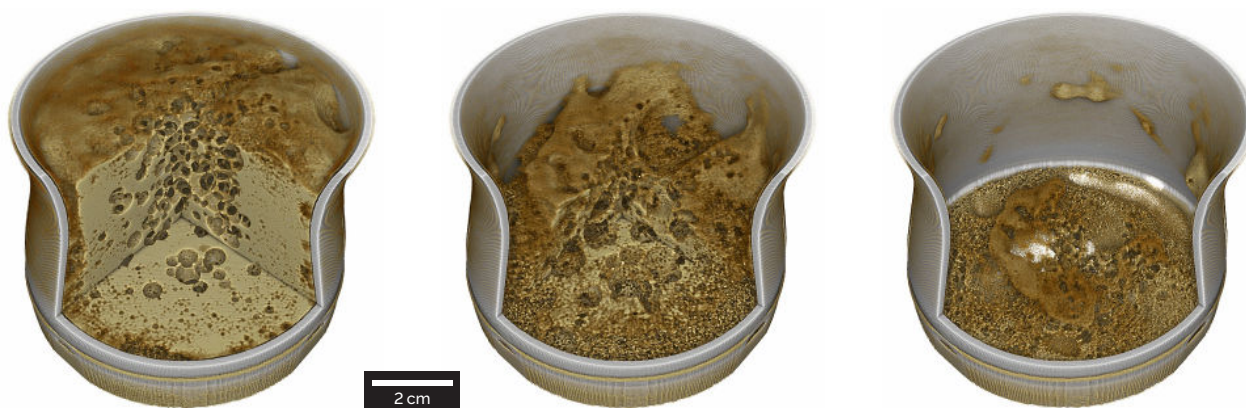
▲ Fig. 2: Evolution of beer foam structure during collapse, showing 3 segments in a continuously acquired dynamic CT series. Temporal resolution: 9 seconds per rotation.
