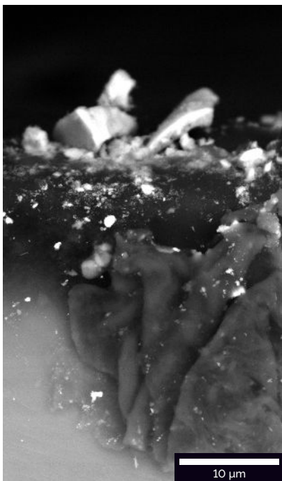
▲ Contamination on the cleaved edge of a display LED (left), contamination and structure of the glass surface (middle) and detail of the tree leaf surface (right). All images acquired in SingleVac mode with chamber BSE detector.
