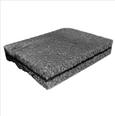
▲ Battery cathode foil imaged at 590 nm voxel resolution
