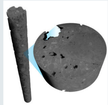
▲ 40 x 3 cm concrete core. 7 mm volume of interest scanned at 5 \mu\text{m} voxel size.
