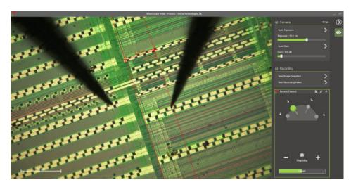
Precisio™ software microscope window with controls for imaging parameters, tools for recording, annotation, and dimensional measuring.
