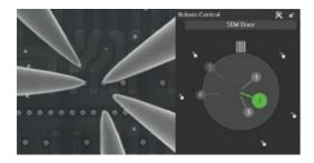
From the main window, the operator is guided through the steps of setting up his nanoprobing system and test recipes, landing probe tips on the device under test, acquiring measurement data and reporting about them.
