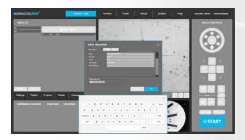
For repeating jobs, IMPRESSIONS™ utilizes the option of setting up and storing custom test programs. For each task, a "job" can be created. All application specific parameters, such as hardness scale, force, dwell-time, pattern, conversion and the report template are stored in the same program.
