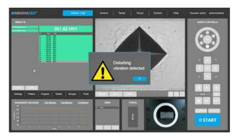
The integrated high precision accelerometer electronics continuously monitor your tester's stability environment. While the tester has vibration isolators (machine dampers) installation environment is often not ideal. Think of heavy traffic, loaded fork lift trucks, excentre presses or other equipment making shop floor installation a base of trouble.
