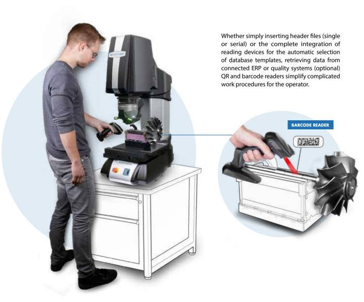
In the above application, a turbo part has been engraved with a QR code. Extra challenging was the fact that the QR code was engraved in a high polished part of the turbo shaft.
