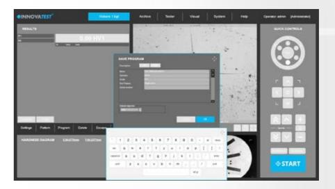
For repeating jobs, IMPRESSIONS<sup>™</sup> utilizes the option of setting up and storing custom test programs. For each task, a "job" can be created. All application specific parameters, such as hardness scale, force, dwell-time, pattern, conversion and the report template are stored in the same program.
