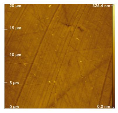
After a 3  $\mu$ m **DiaUltra** step on a Daran cloth the remaining scratches are below 300nm/0.3  $\mu$ m. As the resolution of an optical microscope is about 1  $\mu$ m, these scratches are almost invisible and might only show up in darkfield.
