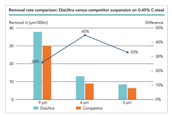
As you can see from this graph, the removal rate of *DiaUltra* is, for all the measured grain sizes, at least 25% higher than the removal of the competitive suspension.
