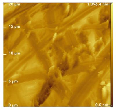
The image to the left shows the surface of a steel sample after fine grinding on an Aka-Allegran 9 with DiaUltra 9 µm. The scratches show a "real" grinding action, where chips are removed in a clean cutting action, with only a very limited amount of deformation. The remaining scratch depth is approximately 1,000 nm/1 µm (see colour scale on right side of image), making it possible to remove the remnant scratches in a short time during the following step.
