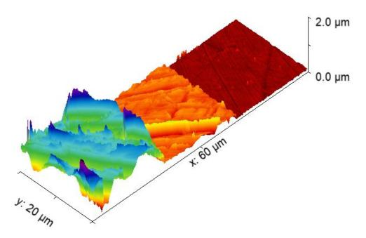
This image combines three different scans after 9, 6 and 3  $\mu$ m preparation steps with **DiaUltra** respectively. It clearly shows how the surface gets finer and finer with shallower scratches after each step.
