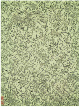
Etial 160 Aluminum Magnification: 100 x
