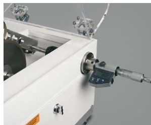
Precise micrometer with digital readout
